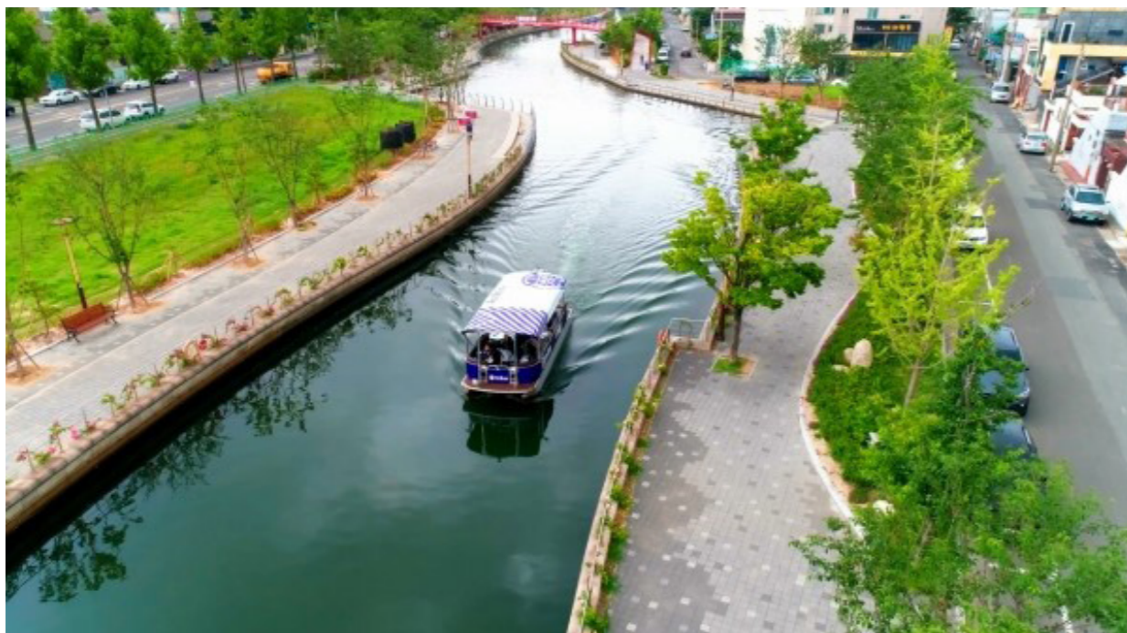
A demonstration of fully autonomous navigation of 12-seater cruise using Avikus' HiNAS/HiBAS conducted at 10km-long Pohang Canal in June 2021
